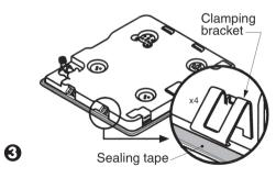
3 Place hotplate on top of the bench cut-out and press down firmly on all edges at the same time to ensure that the hob is resting on its entire perimeter.
